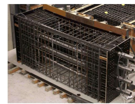
Mock-up before concreting
