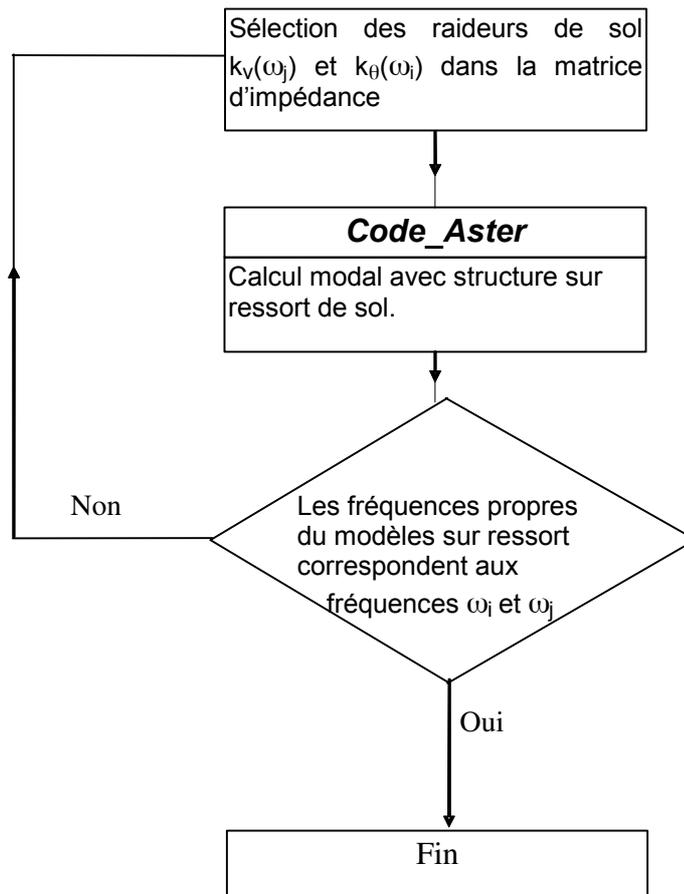
Figure 6.1-a : Process of adjustment of the stiffnesses of ground.
