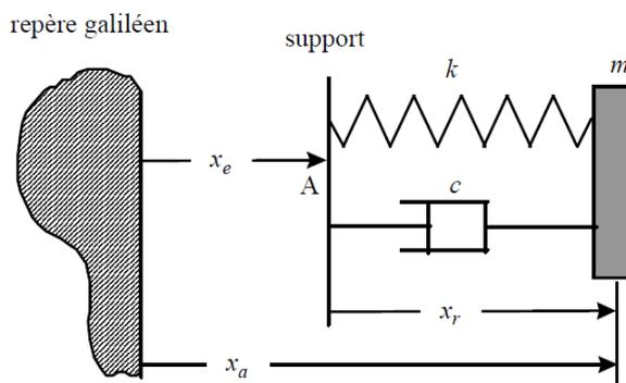
Figure 2-a : simple oscillator subjected to a seismic request.
