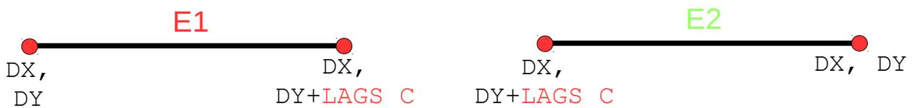
Figure 12: Attribution of the degrees of freedom on the meshes of contact slave SEG2/TRIA3
