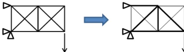
Figure 3.5-a: Optimization of sections. Reduction of section of the elements
