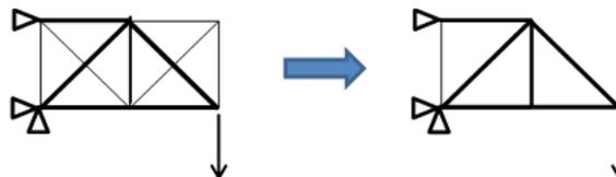
Figure 3.5-b: Topological optimization. Elimination of elements
