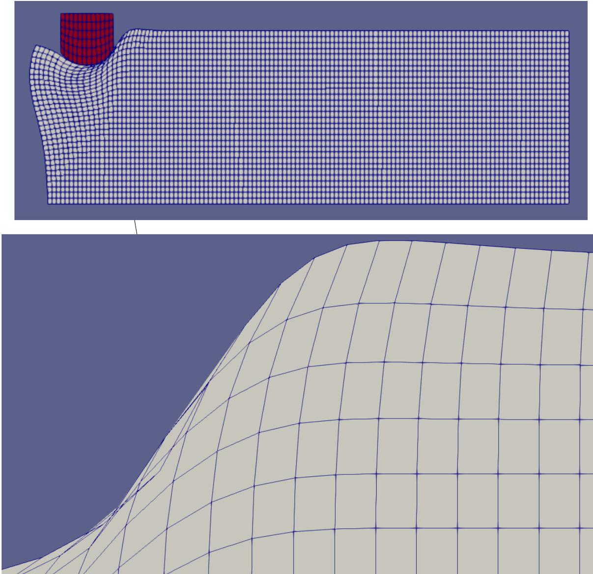
**Figure 4.1-1: Situation of turned over mesh leading to the failure integration of the law of behavior**
