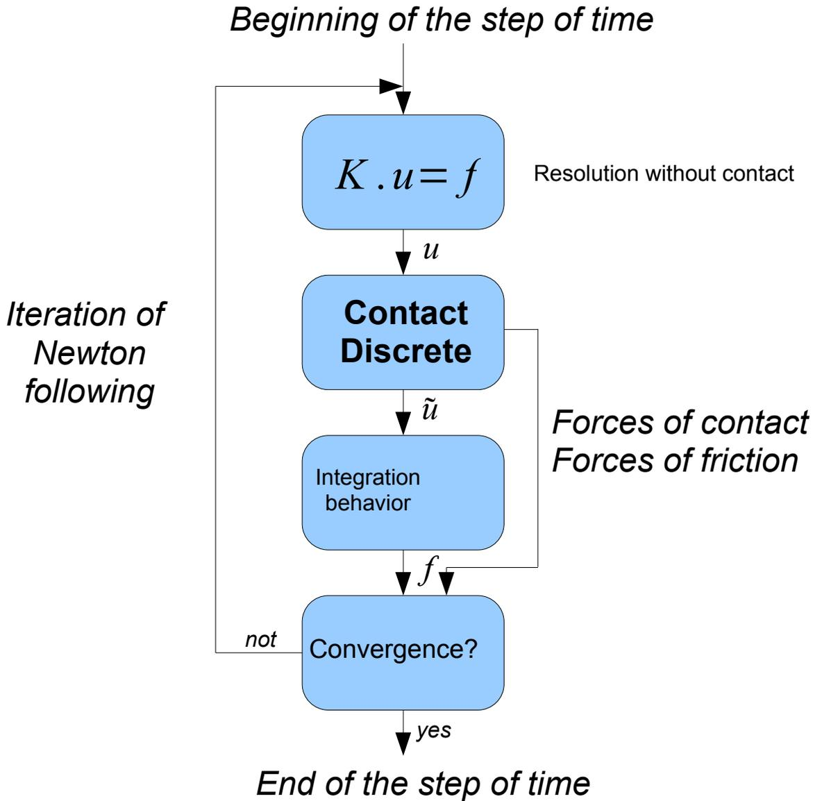
Figure 3.1.2-1: Algorithm general of a step of time in discrete formulation (small slips)
