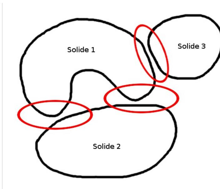
Figure 2.1-1: Definition of three zones of contact
