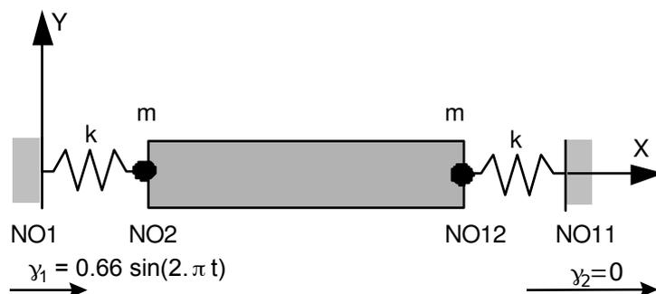
Figure 3.1-a: Modeling of the seismic anti device
