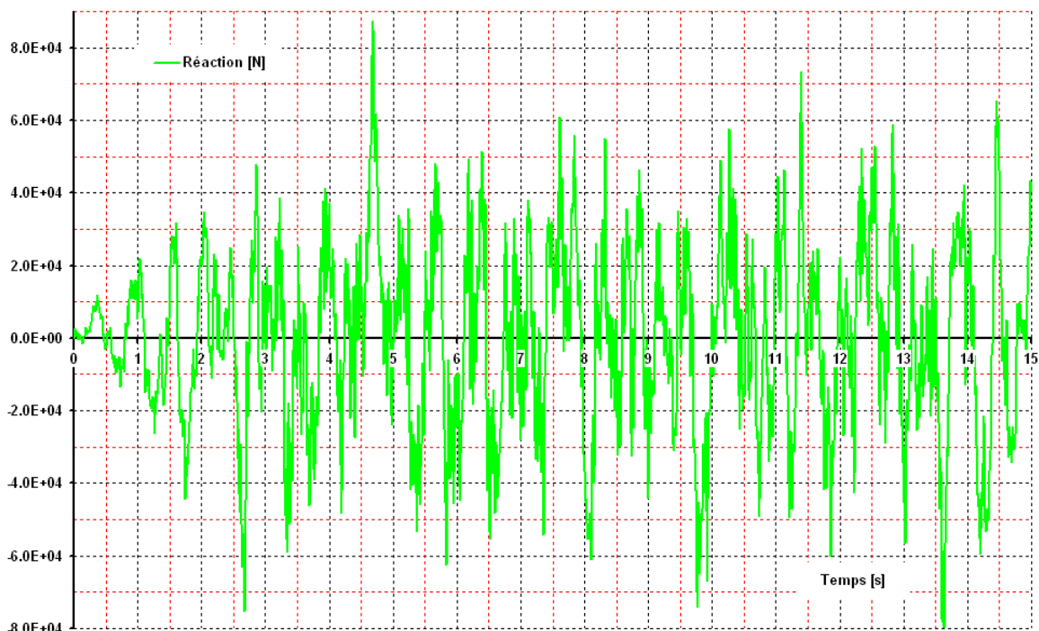
Figure 3.2-d : Réaction of support in A according to time, for 15 seconds.
