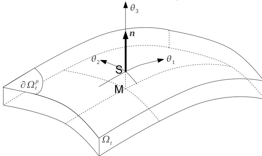
**Figure 2-3: Curvilinear parameter setting of the vicinity of the surface subjected to the pressure**
