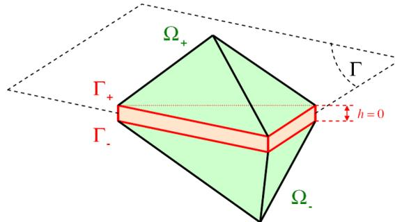
**Appear 2.3-a : Discretization by finite element of interface.**
