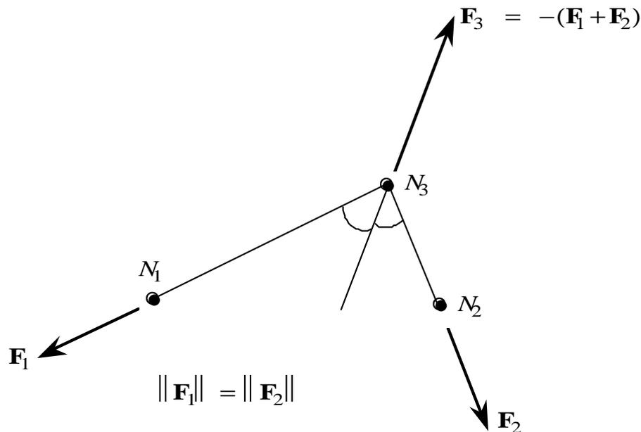
Figure 4-a: Internal forces of an element of cable-pulley
