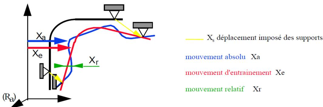
The absolute displacement of any point *M* of structure, not subjected to an imposed displacement, is equal to the sum of relative displacement and the displacement of training of this point:
