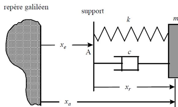
Appear 2-a : simple oscillator subjected to a seismic request
