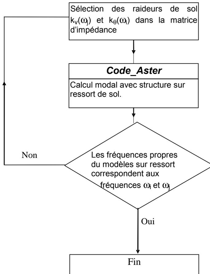
Appear 6.1-a : Process of adjustment of the soil stiffness
