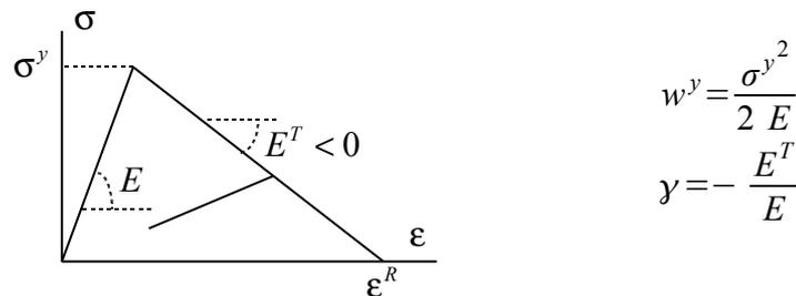
Figure 2.2-a: Simulation of a traction test simple
