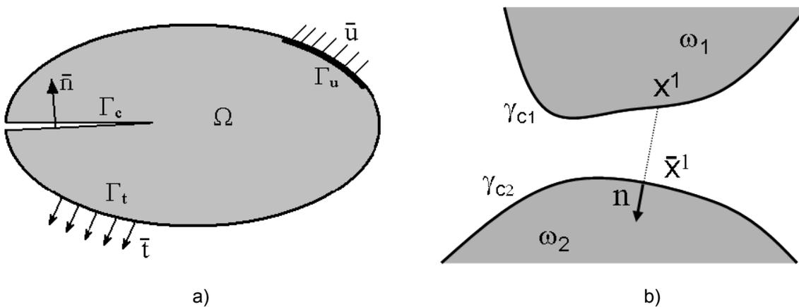
Figure 2. a) Notation of the problem of contact; b) Evaluating of clearance enters the point of contact and its project.
