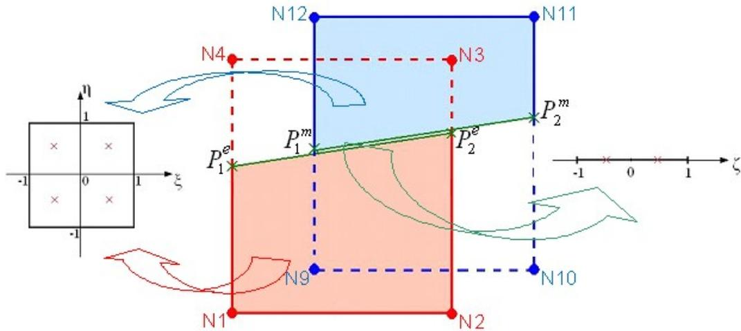
Figure 4. Hybrid example of element of contact great slidings X-FEM.
