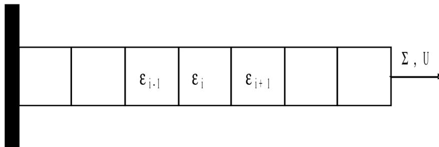
Appear 2-a: Assembly of identical elements assembled in series subjected to a traction test
