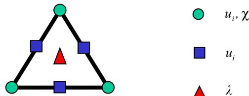
Appear **2.3-a** : Discretization finite element of the model second gradient of thermal expansion for the plane strains
