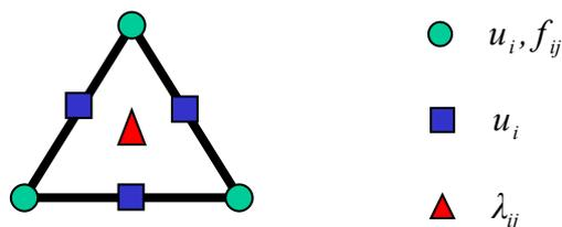
Appear **1.3-a** : Discretization finite element of the model second gradient for the plane strains
