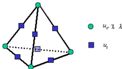
Appear **2.3-b** : Discretization finite element of the model second gradient of thermal expansion for 3D.
