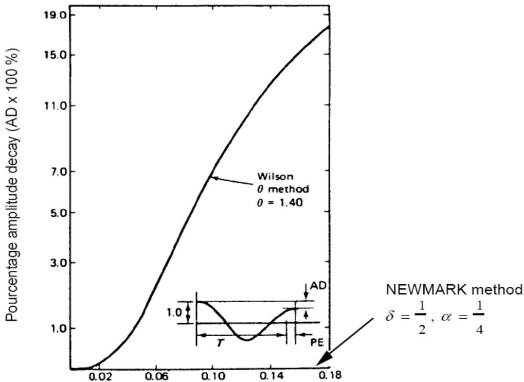
It is checked here that the algorithm of NEWMARK with these parameters does not present any numerical damping.
