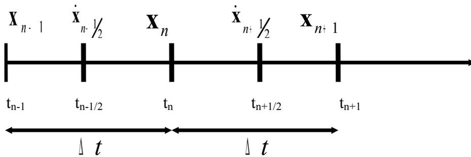
The velocity is expressed with indices half-integers of the discretization in time whereas displacements and accelerations are expressed with the whole indices. Written this way, the diagram is of order 2.
