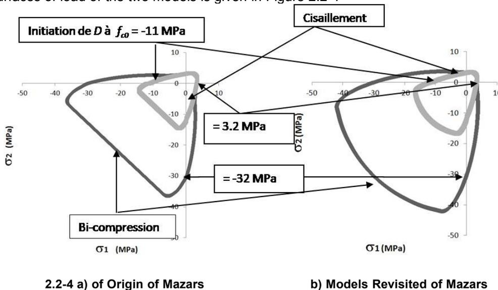
Figure 2.2-1 : Comparison of surfaces of initiation of damage and fracture of the Mazars models in the plane  $\sigma_3 = 0$  and a concrete C30
