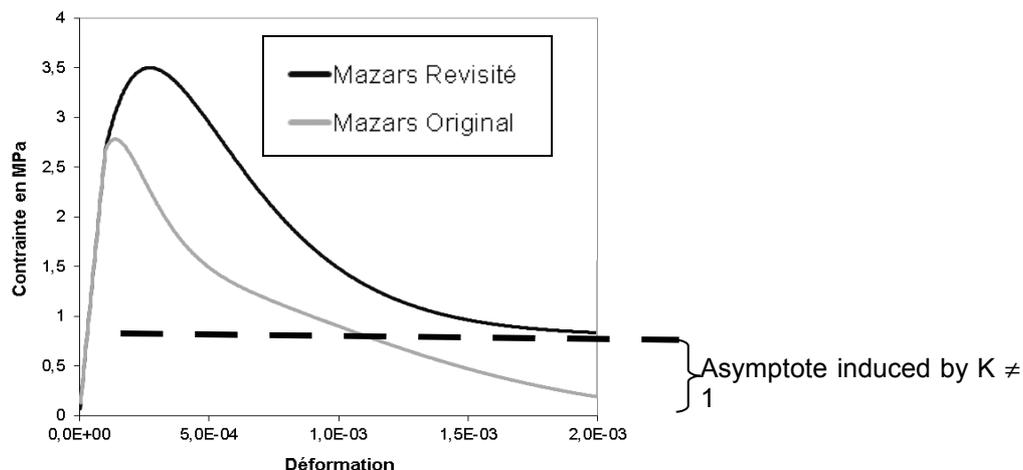
**Figure 2.2-3 : Stress-strain curve during a test of pure shears on a Gauss point**
