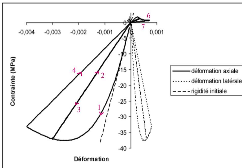
**Figure 2.2-4 : Response stress-strain of the model of Mazars for a request 1D.**
