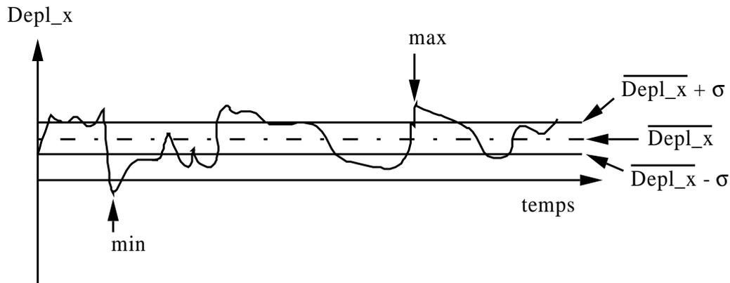
**Appear 3.2-a: Example of signal of displacement and visualization of the statistical quantities**
