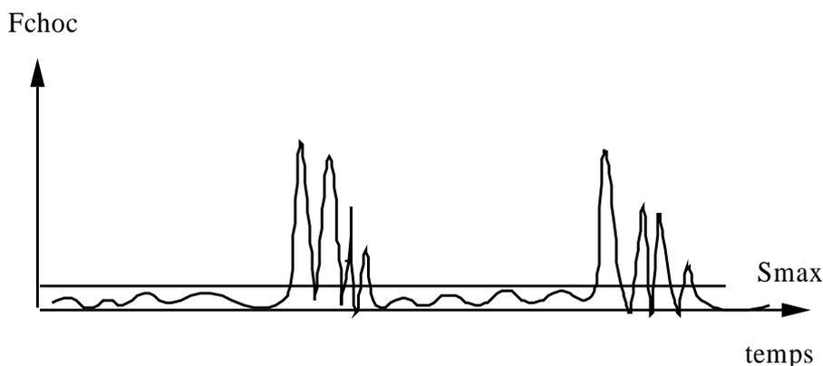
Appear 3.3-a: Example of experimental signal of shock force
