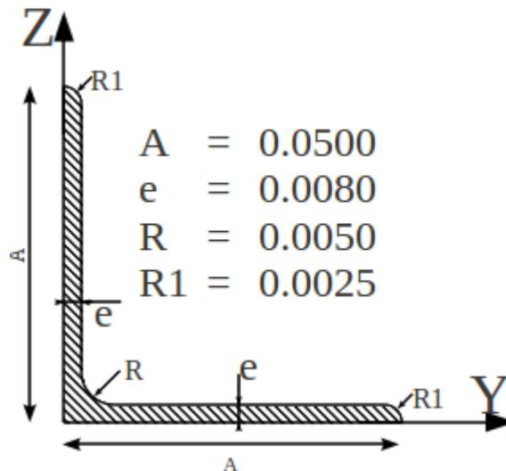
Figure : Angle with equal wings 50x50x8.
