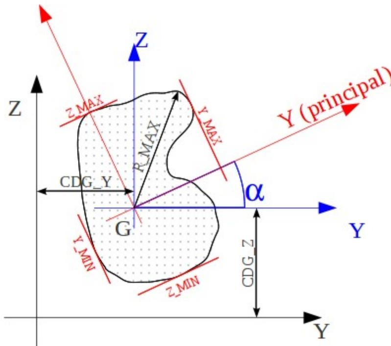
Appear 3.1-a Definition of the geometrical magnitudes relative to a section of beam.
