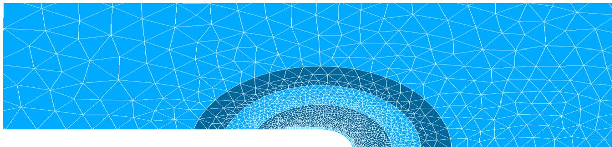
Figure 3-3 - Free mesh without definition of the chips.
