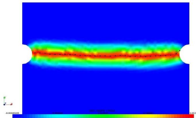
Figure 4.2-1: way of cracking in the bi-notched test-tube (model ENDO\_SCALEIRE).
