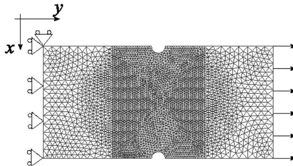
Figure 3.1-1: geometry, mesh and boundary conditions of the tensile specimen.
