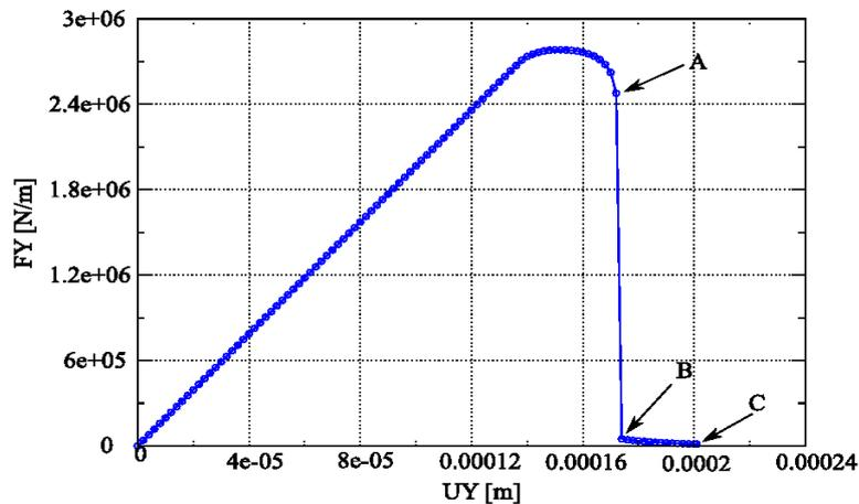
Figure 5.1-1: Curve force-displacement, bi-notched test-tube (model MAZARS).
