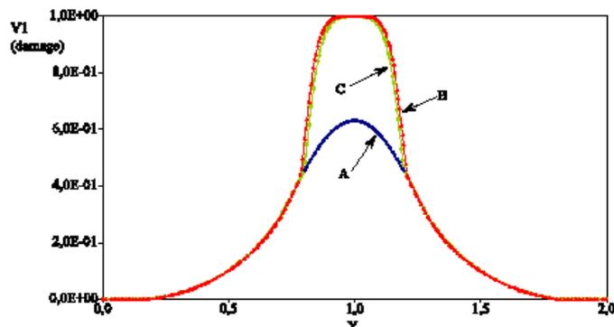
Figure 5.1-3: Damage on the longitudinal axis of the test-tube (model MAZARS).
