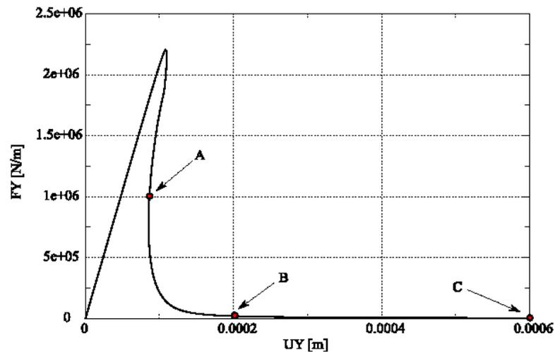
Figure 4.1-1: Curve force-displacement, bi-notched test-tube (model ENDO\_SCALEIRE).
