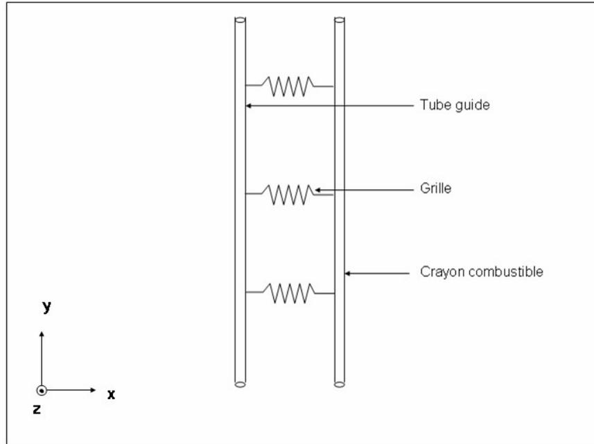
the geometry is a fuel pin height  $4,5\text{ m}$ , thickness  $0,5\text{ mm}$  and diameter  $0,9\text{ cm}$ , regularly attached, via the grids of maintenance, with a tube guides, more rigid, of thickness  $0,5\text{ mm}$  and diameter  $1,245\text{ cm}$ .
