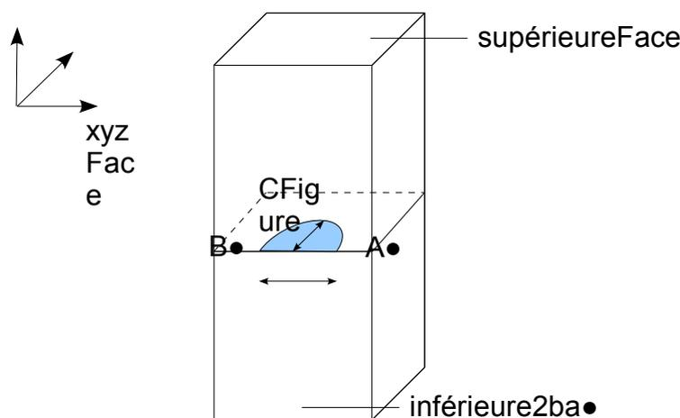
1.1-1: Geometry of initial crack
