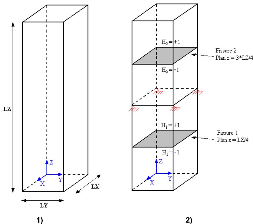
Figure 1.1. Geometry of the bar and positioning of crack
