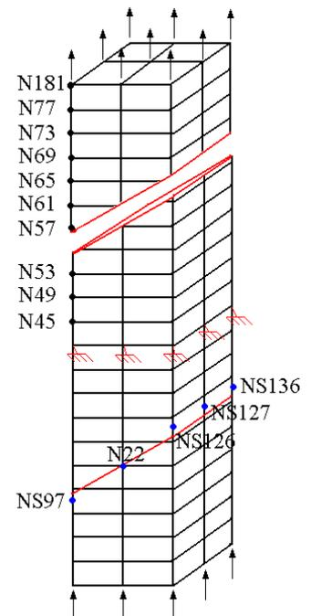
Figure 4.4-1: Final mesh and positioning of the nodes tested
