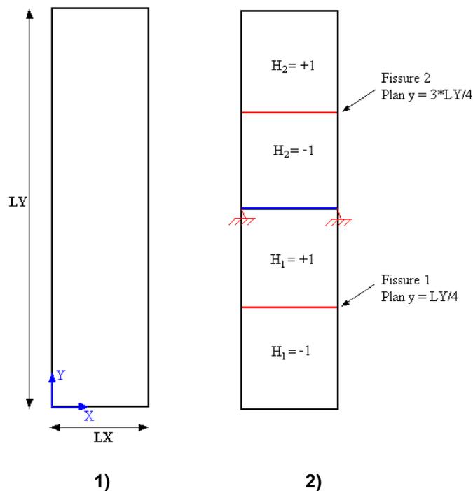
Figure 1.2. Geometry of the plate and positioning of the crack
