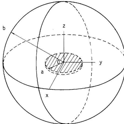
a: radius of crack interns circular in the horizontal plane xoy
