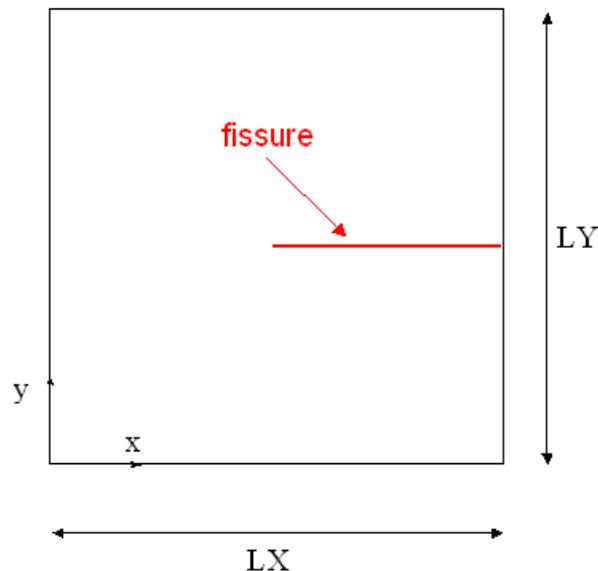
Figure 1.1-1 : geometry of the fissured square plate
