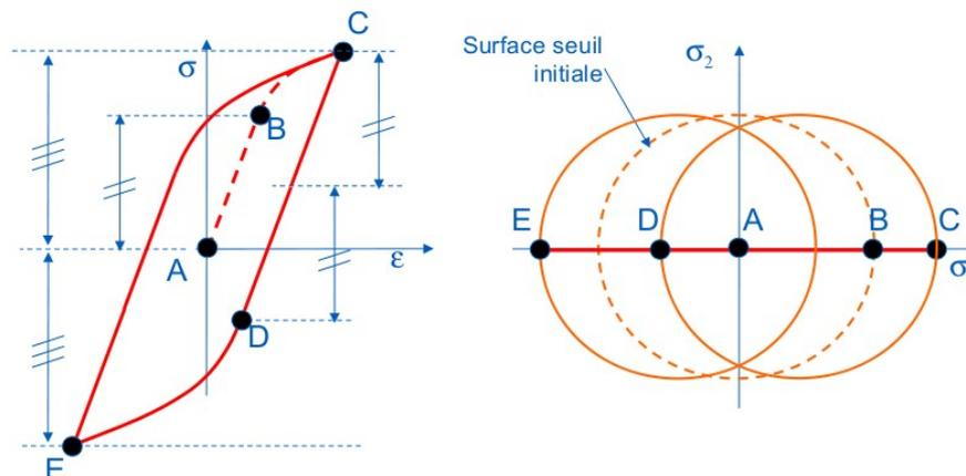
Figure 1.8-2 : Kinematic work hardening
