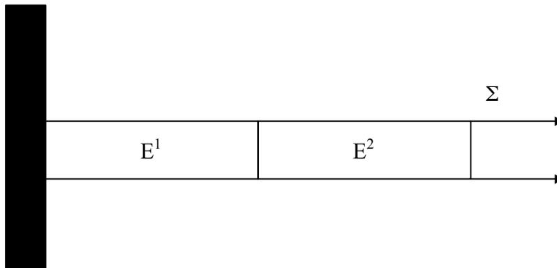
On the interface between the two elements, the discontinuity of modulus Young thus imposes a discontinuity of the deformation. Let us consider now either the local deformation but a delocalized deformation. The classical operators of delocalization cause to return continues the deformation in the structure, which then generates obligatorily a discontinuity of constraint to the interface because of the difference of Young modulus, and this goes against the equilibrium equation.
