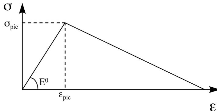
Figure 2-b: Law of behavior of material in uniaxial simple traction
