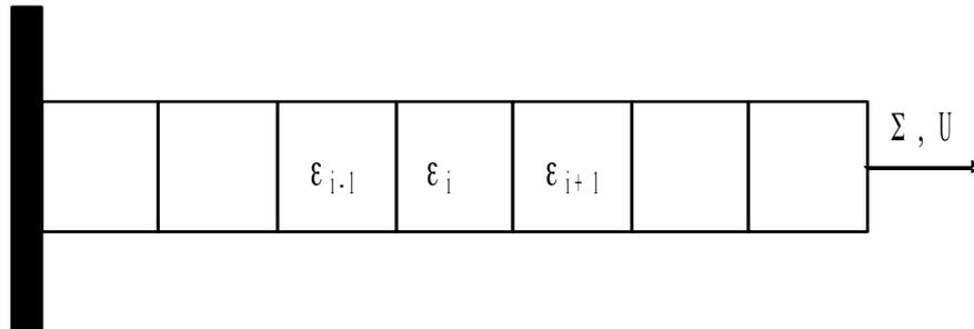
Figure 2-a: Assembly of identical elements assembled in series subjected to a tensile test
