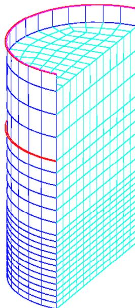
Figure 4.1- has: Complete grid with the fluid field and the structure
