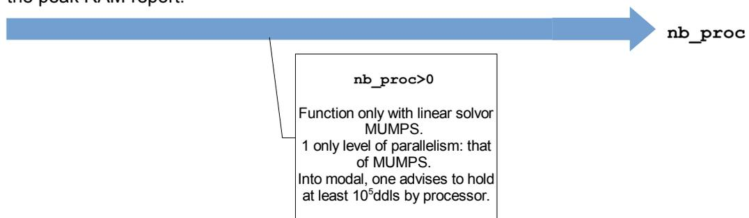
Image 3.12-3 - Perimeter of use with `NIVEAU_PARALLELISME='PARTIEL'`.
