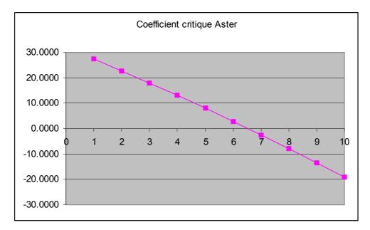
In elastoplasticity, one tests the moments when the critical coefficient changes sign. The tests are of nonregression since one does not have analytical solution in this case.
