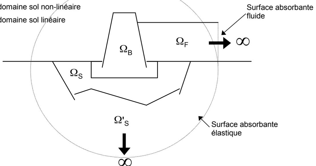
Figure 1.1-a: Field for the interaction ground-fluid-structure
