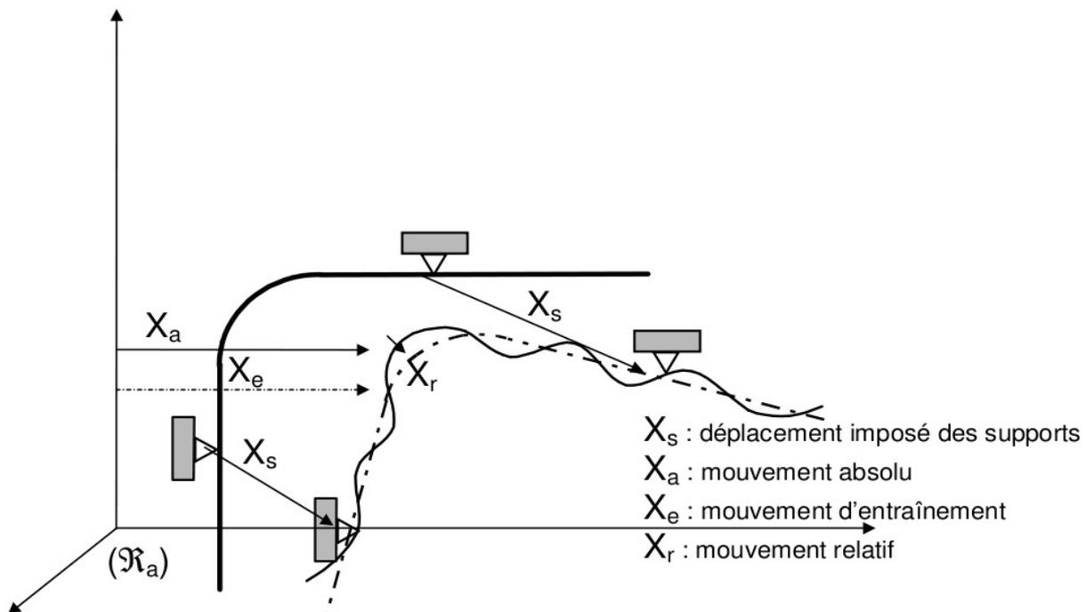
Figure 4.1-a: Decomposition of the movement of the structures
