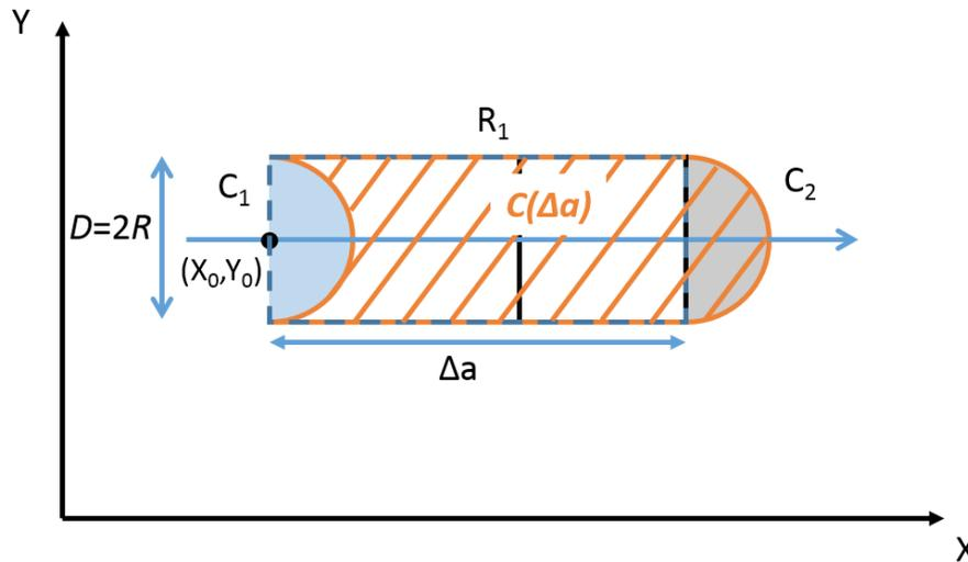
**Figure 2-b – Definition geometrical of the notch: the zone  $C(\Delta a)$  in hatched, the rectangle  $R_1$  in dotted line, and half-discs  $C_1$  and  $C_2$ .**
