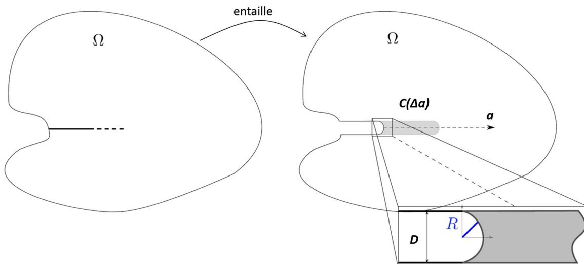
Figure 2-a – Modeling DU defect by a notch and representation of the zone of virtual propagation  $C(\Delta a)$  in gray.
