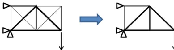
Figure 3.5-b: Topological optimization. Elimination of elements
