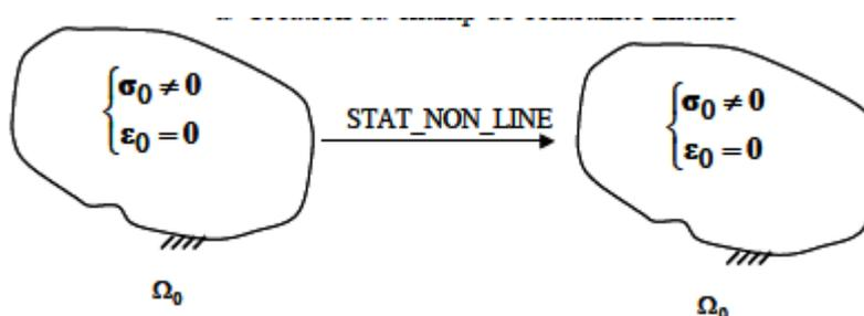
Figure 3.1 : Checking of the validity of the initial stress field.
